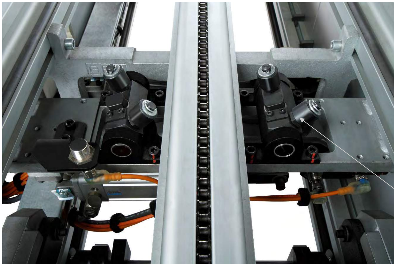
Synchronised rockers with one stopping and one isolating roller each
